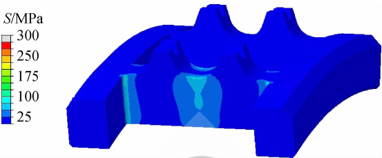
图 13 兜孔圆角 R=0.1\text{ mm} ,100 N 作用力情况下应力值 Fig. 13 Value of stress when pocket fillet R=0.1\text{ mm} , the force is 100 N
